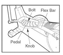
pedal forward or backward to the desired position, and then retighten the knob. Make sure that both pedals are in the same position.
